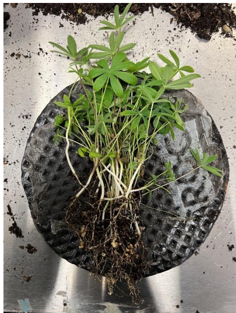
Showing root development of top of Proofex Torchseal A700, but no root penetration through barrier
