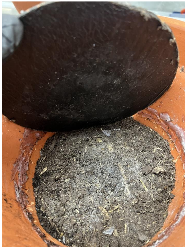
Showing root development of top of Proofex Torchseal A700, but no root penetration through barrier
