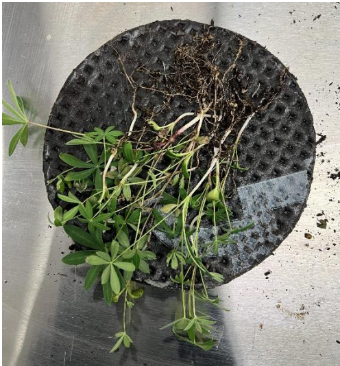
Showing root development of top of Proofex Torchseal A700, but no root penetration through barrier
