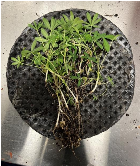
Showing root development of top of Proofex Torchseal A700, but no root penetration through barrier
