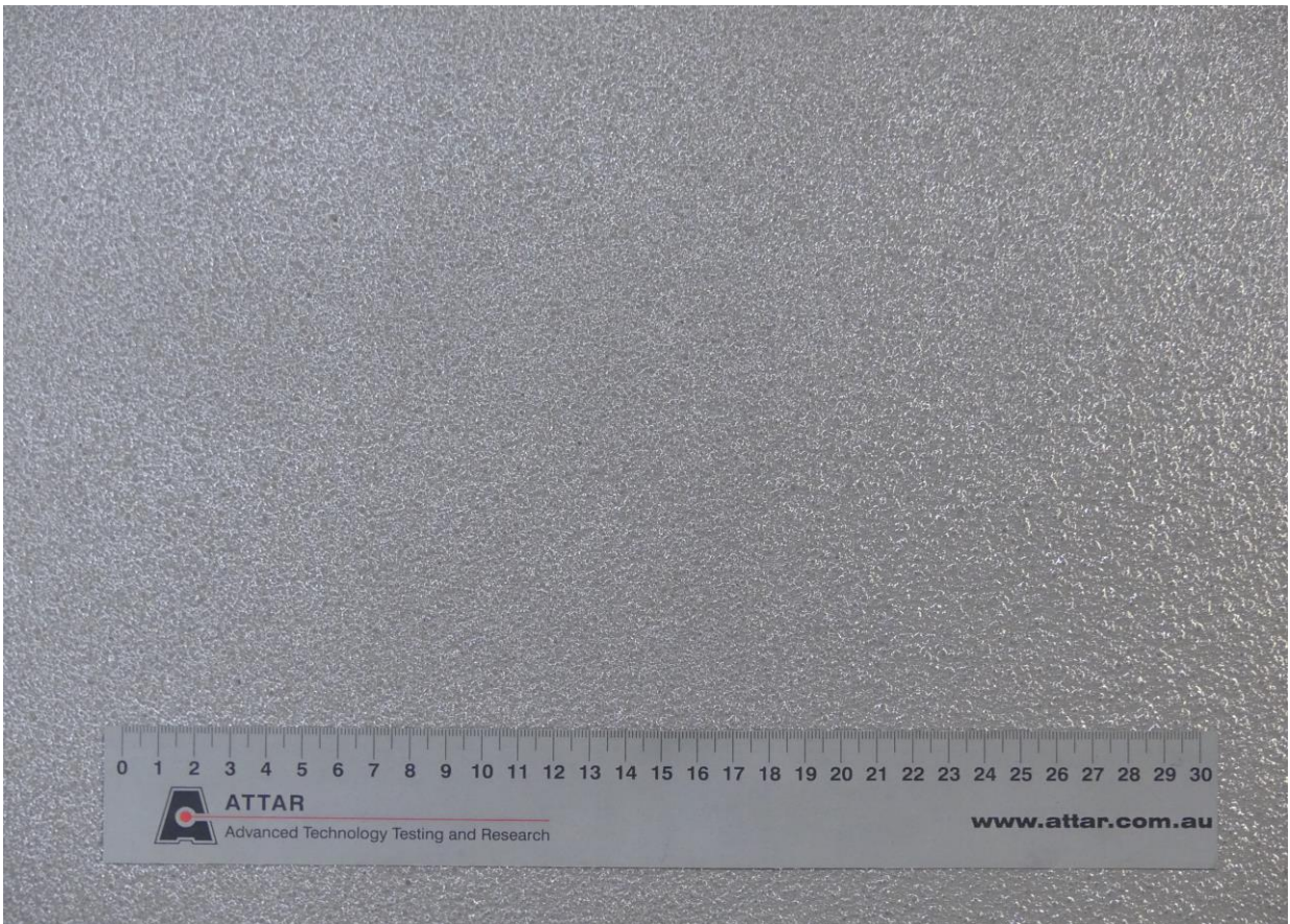
Figure 1: Fosroc Nitoflor FC150 HP-FC + Fosroc Nitoflor Anti-Slip Grains 02 Silica Sand 30/60# + Fosroc Nitoflor FC150 HP-FC
