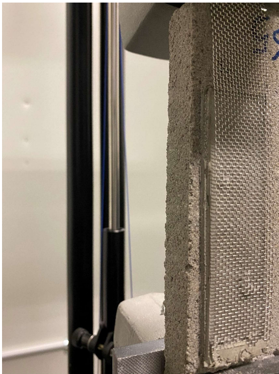
FIGURE 4 IMAGES OF TEST SAMPLE PERFORMING ADHESION-IN-PEEL
