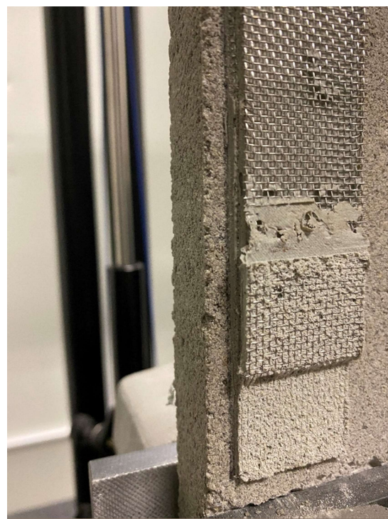
FIGURE 4 IMAGES OF TEST SAMPLE PERFORMING ADHESION-IN-PEEL
